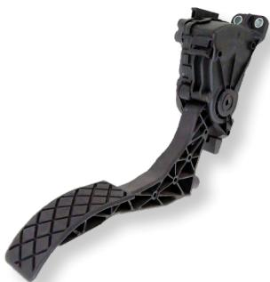
The accelerator pedal position sensor is an **electronic device that detects the position of the accelerator pedal** by detecting the pressure applied by the driver and transmitting this data to the engine control unit (ECU). The ECU **adjusts the amount of fuel injected** and the throttle opening, thereby enabling **effective management** of engine torque, fuel consumption, and pollutant emissions.
