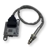
The NOx sensor measures the concentration of nitrogen oxides (NO and NOx) in exhaust gases in real time. These gases are major pollutants produced by internal combustion engines, especially at high temperatures. The data collected by the sensor is transmitted to the ECU, which then adjusts the pollution control system (by injecting AdBlue®) to reduce NOx emissions.
