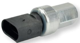
The air conditioning pressure sensor is an essential component in a vehicle's air conditioning management system. It **measures the pressure of the refrigerant in the circuit to ensure optimum operation of the air conditioning system**. This sensor is designed to protect the system by regulating pressures that are too high or too low, and by enabling certain circuit components to be switched on or off.
