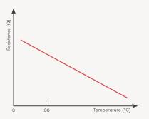
How NTC (Negative Temperature Coefficient) technology works: as the temperature rises, the value of the resistor decreases. The higher the temperature, the lower the resistance.
