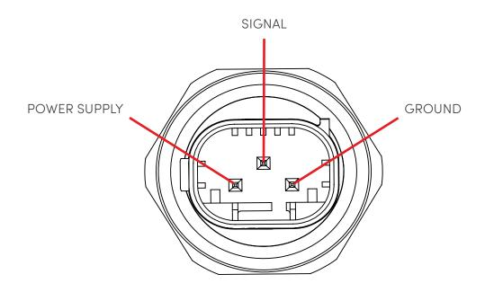
Caution! Remember to position the connector in the right direction (with the keyed connection downwards).
