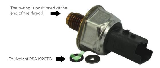
Before fitting, check that there is a washer in the injection rail: if a washer is already in place, replace it with the one supplied in the box with the sensor. On the other hand, if no washer is present, do not add the one supplied.
