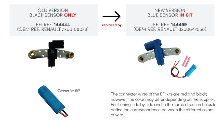
The colour of the wires in the engine beam differs from one vehicle to another. For example, on Kangoo, the wires are green and pink; on Twingo, they are white and green; and on Clio, they are orange and white. Pay attention to the correct match with the wires of the connector.
